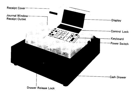
Power Switch ... The Power Switch is located at the righthand side of the cabinet. The AC power is turned on when the switch is pushed to ON, and turned off when the switch is pushed to OFF.
